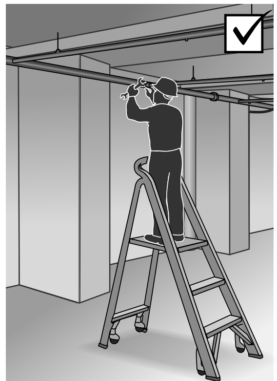
Figure 24 Solution: a step platform provides a stable work surface
