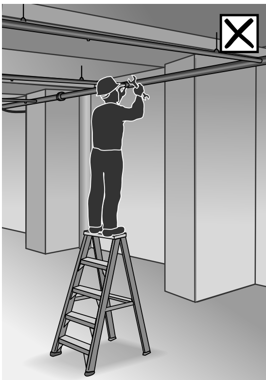
Figure 23 Hazard: standing above second tread of a stepladder
