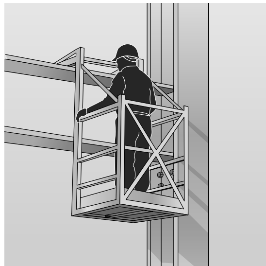
Figure 6 Fabricated hung scaffold – purpose-designed temporary structures that are anchored to a permanent structure to support a working platform
