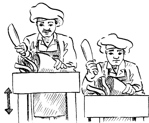
After: Adjustable work heights allow the butchers to set the bench to suit their height and task. Bending is reduced for the taller employee, and the need to work with raised arms is minimised for the shorter employee.
