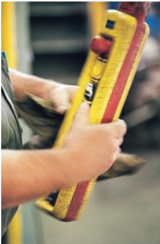
Remote control device that allows an operator to work at a distance away from a noise source
