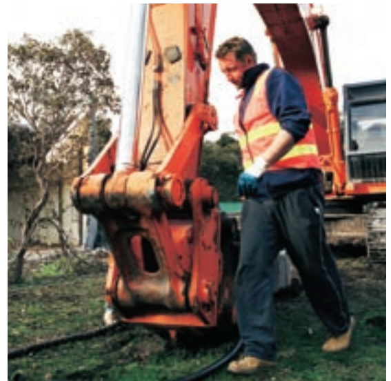
Working near a front end loader generally involves a significant amount of noise that may be above the exposure standard
