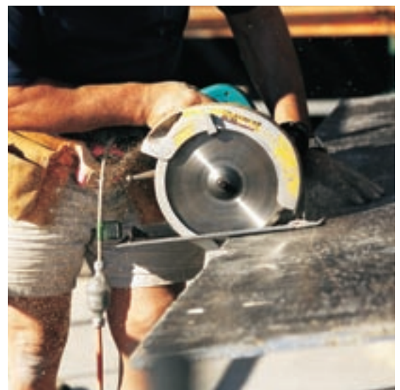
If cutting with a circular saw is required, the material being cut will determine the amount of noise produced
