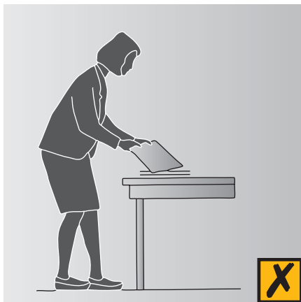
Figure 4.8 Incorrect standing-height bench
