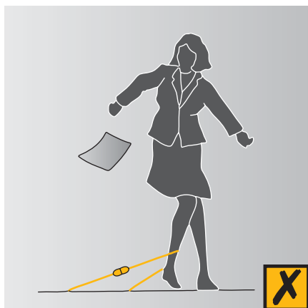
Figure 6.3 Electrical and trip hazards
