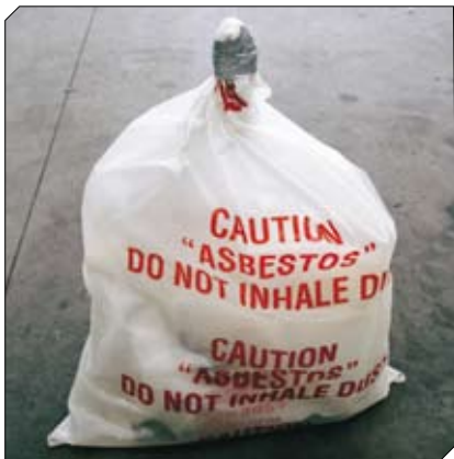
Figure 8: An asbestos waste bag with appropriate warnings.
