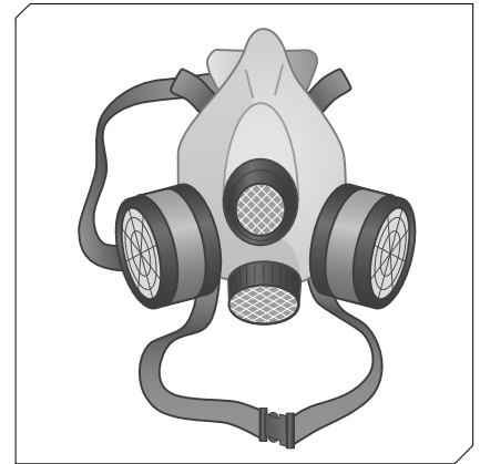
(B) Half-face, particulate filter (cartridge) respirator.
