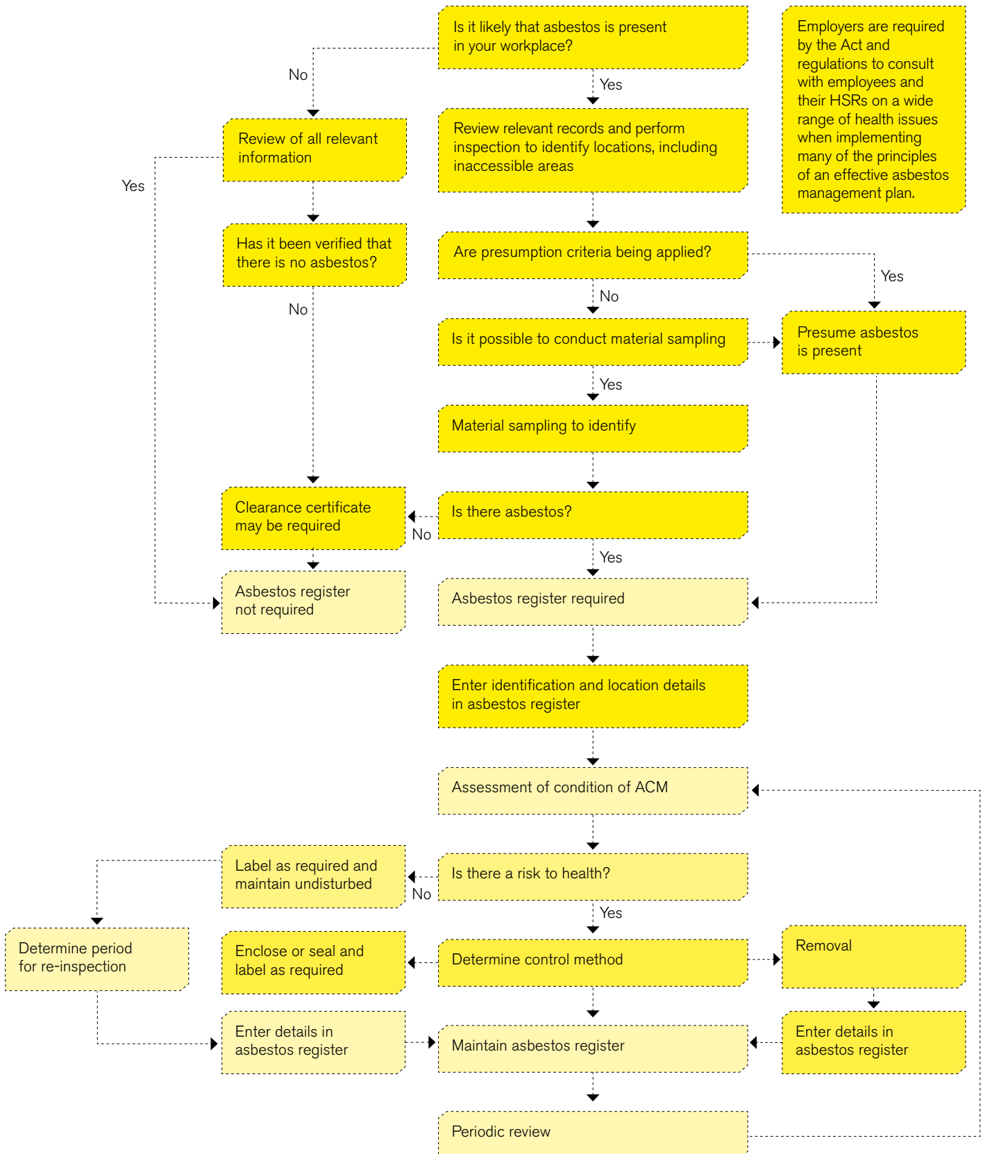
Diagram 1: General principles of an asbestos management plan
