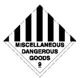
The Class label must not be less than 250 mm square and must be firmly affixed to the vehicle.
